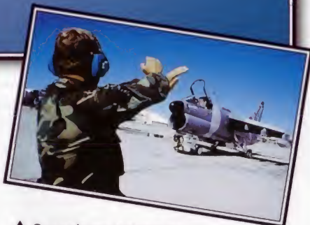
▲ Groundcrew prepare an A-7 for a training mission. The naval origins of the aircraft are given away by its strong main landing gear and long nosewheel strut.
